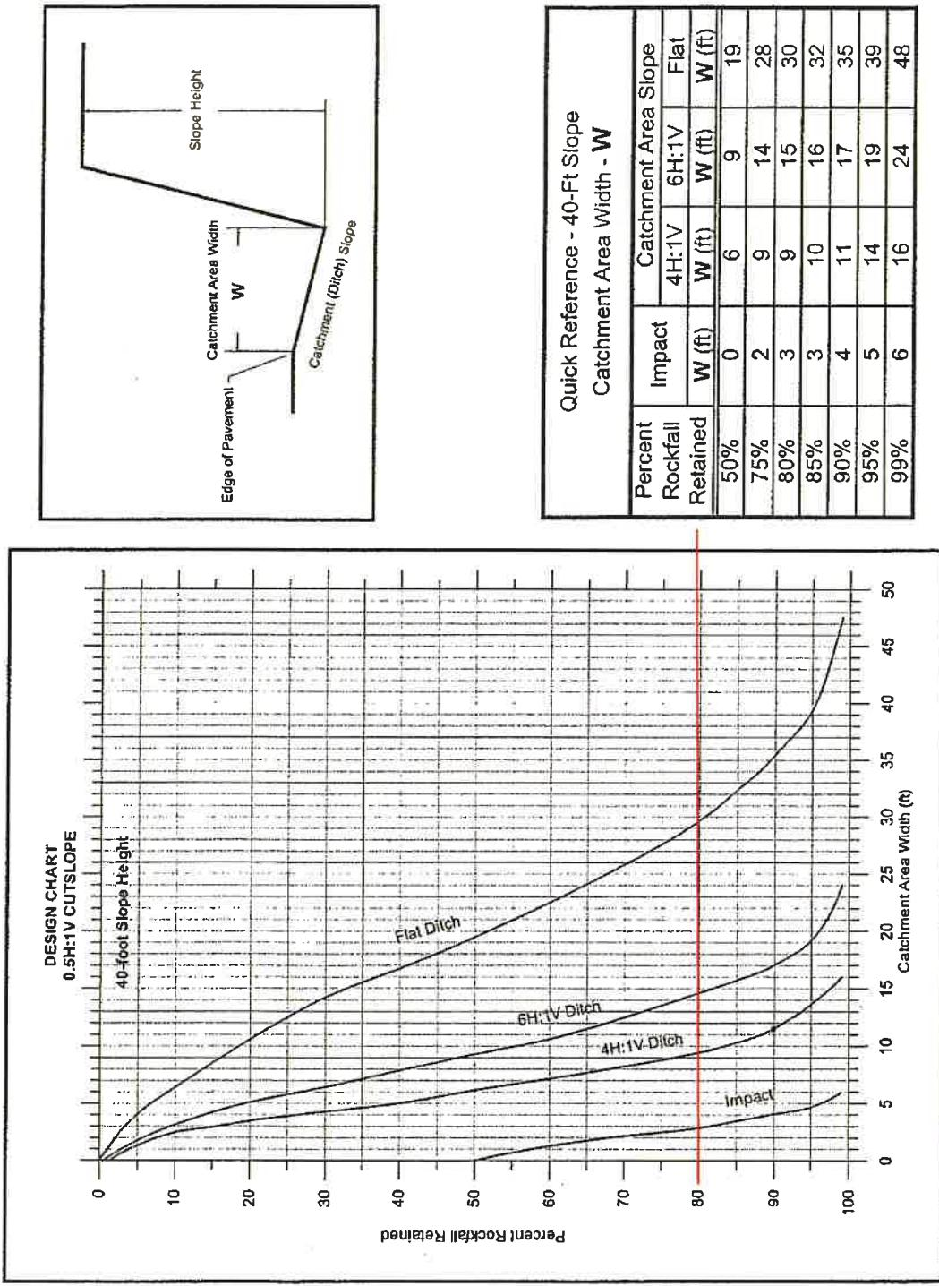
Figure 5.11: Design chart for 40-foot high 0.5H:1V cutslopes
