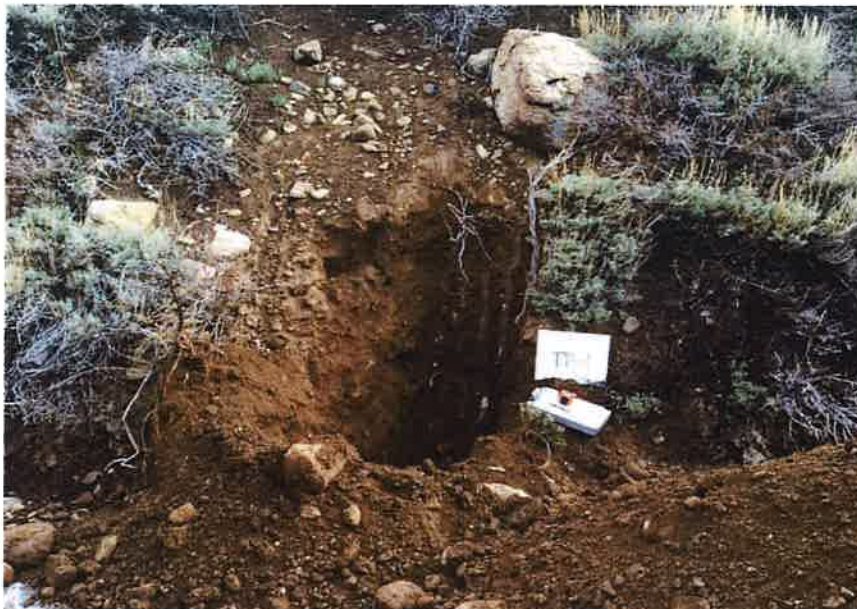
Photograph 44. Test Pit TP-1 during excavation.
